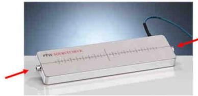
Fig1. Cámara SourceCheck, PTW
